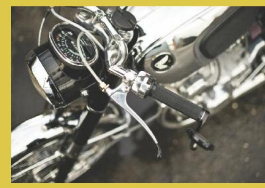
ignition, and the charging was improved with his single unit regulator/rectifier. He also upgraded the coil to a 30,000 volt 3 ohm Dynatek mini coil, which he uses exclusively. All controls are original, as in his opinion they are beautifully designed and can always be repaired and cleaned up. The rear-sets were fabricated from old parts from his stash. "I think that the fit and function are very nice, if I do say so myself. The
